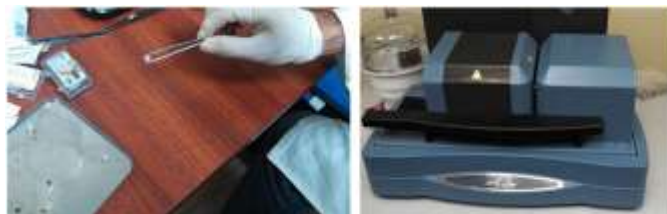
Figure 7.- Sample placement for TGA analysis.
