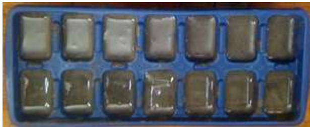
Figure 1.- fly-ash based geopolymer pastes.
