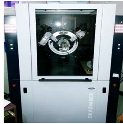
Figure 2.- X-ray diffractometer D8 Advance, brand: Bruker.
