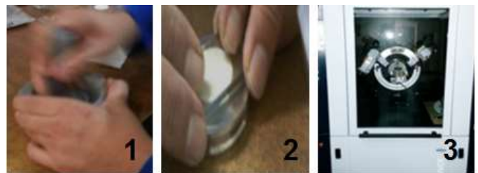
Figure 4.- Sample preparation procedure for X-ray diffractometer.
