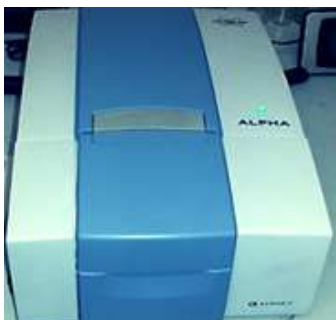
Figure 5.- infrared spectroscopy equipment, FTIR- Alpha 1, brand: Bruker.
