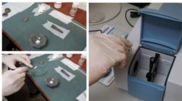
Figure 6.- Sample preparation procedure for FTIR.
