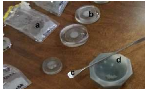
Figure 3.- Minor equipment and sample preparation in X-ray diffractometer instrument; a) geopolymer sample, b) sample holder, c) spatula d) agate mortar and spatula.
