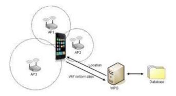
Figure 2. Structure of Wi-Fi positioning system
