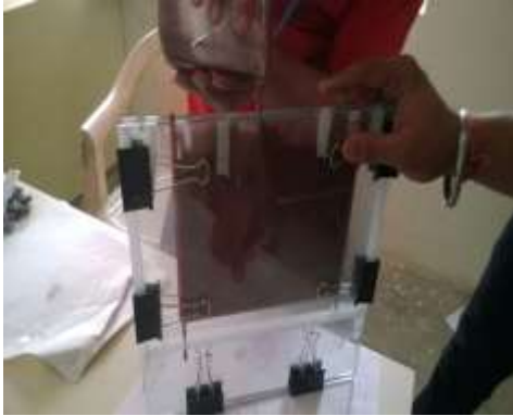
Figure 3. Pouring of Mixture in the Mould
