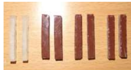
Figure 5. Specimens for 2-body wear test
