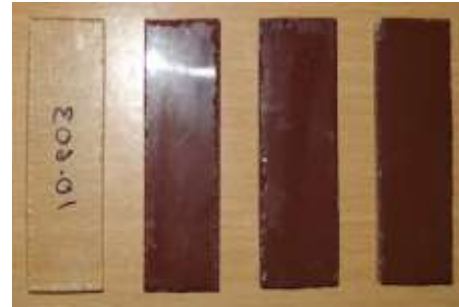
Figure 7. Specimen for 3-body wear test
