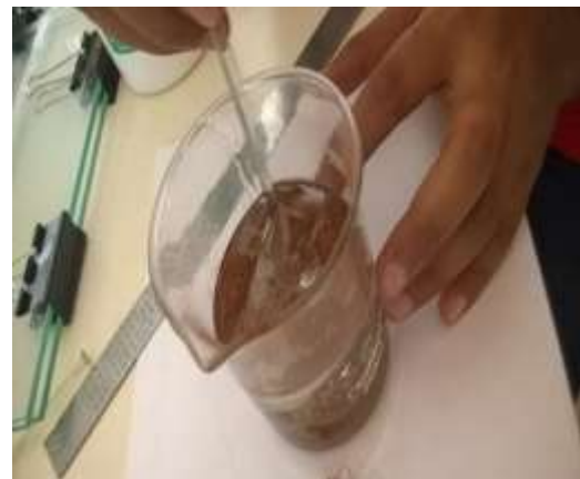
Figure 2. Mixing Epoxy-Copper with Hardener
