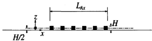
b) Side view of the aligned array configuration
