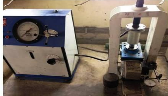
Figure 2. Experimental set up for deflection and displacement assessment
