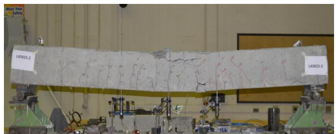
Figure 5. Mode of failure for beam L45R25-2
