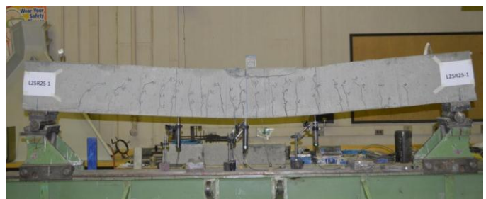
Figure 4. Mode of failure for beam L25R25-1
