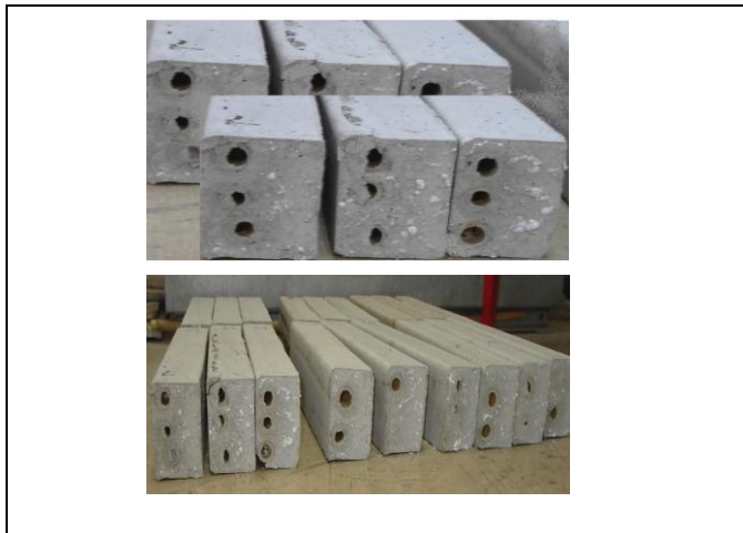
Figure 2. Specimens for compression (above) and flexural (below) tests.
