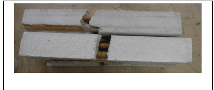
Figure 3. Displacement of the reeds produced due to a bad adhesion
