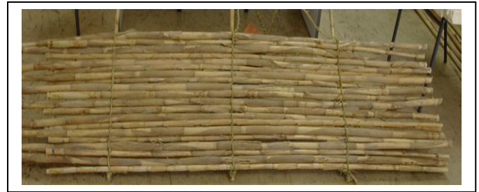
Figure 1. A piece of a mat made of culms of Arundo donax L.
