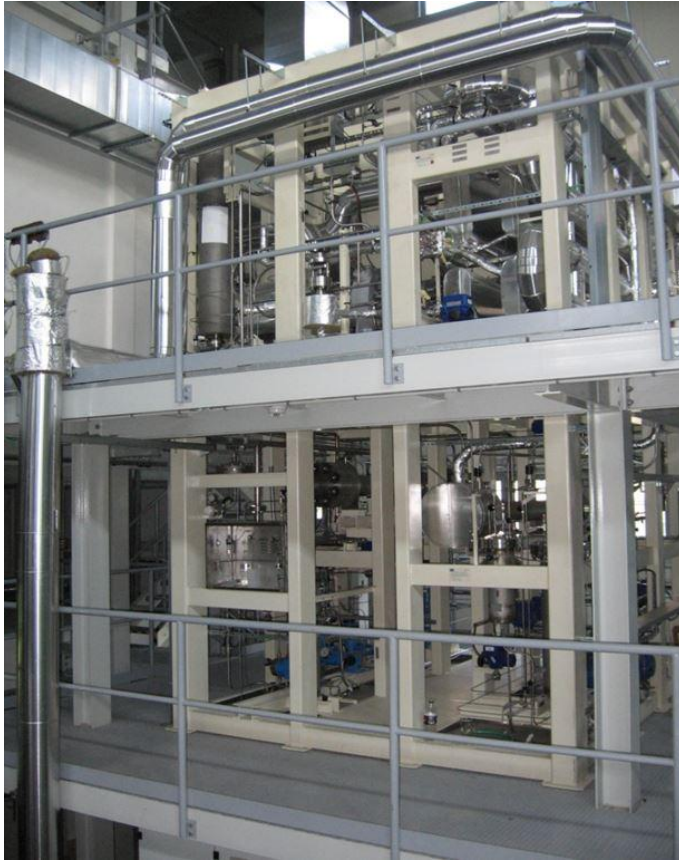
Figure 1. Supercritical water loop in Research Centre Rež. Active channel (vertical pipe in the very left is still in out-of-pile operation)
