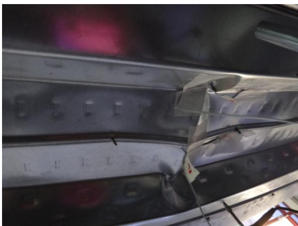
Figure 5 Local buckling for CS sample
