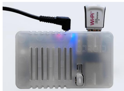
Figure 2. ODROID-U3 as a DETIboot server.
