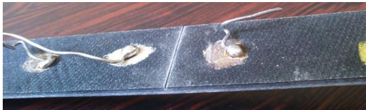
Figure 2: Photograph of a specimen with a formed artificial notch and electrical cable connectors
