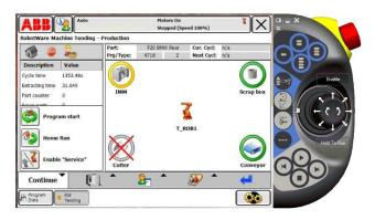
Figure 3 Flex-Pendant interface for machine tending
