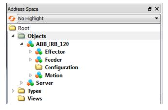
Figure 6 Screenshot of an OPC UA client showing the server's address space
