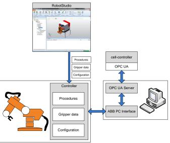
Figure 5 OPC UA server for ABB machine tending robots
