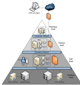
Figure 4 OPC UA as communication interface in the Automation Pyramid
