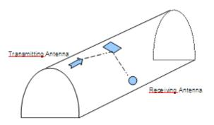
the sum of each contribute resulting from scattering of every incident EM waves on tunnel surface and directed towards the receiver antenna.
