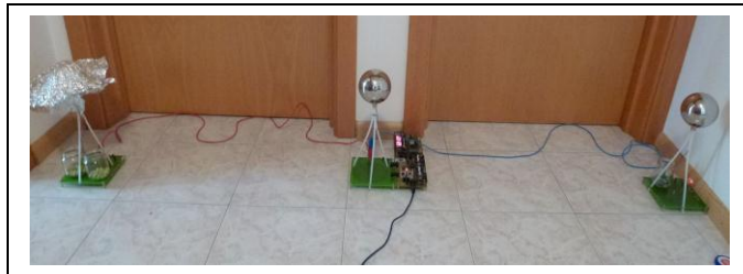
Fig. 6 Positioning of power-transmitter (center), the first receiver (left) with the pea seeds to be treated and the second receiver (right) with the gibberellic acid as information source (or the apoptosis signal emitting peas, respectively).
