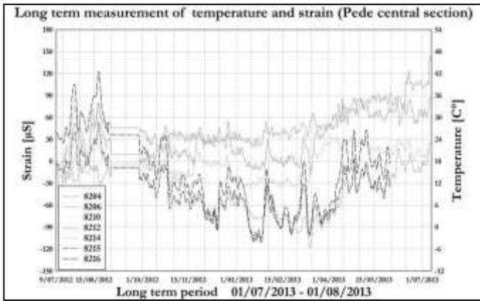
Figure 5. Long-term measurement graph of temperature and strain
