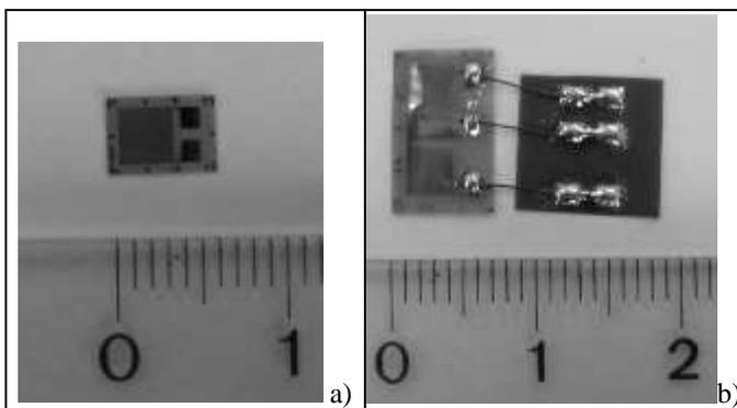
Figure 3 a) Temperature sensor; b) Strain gauges
