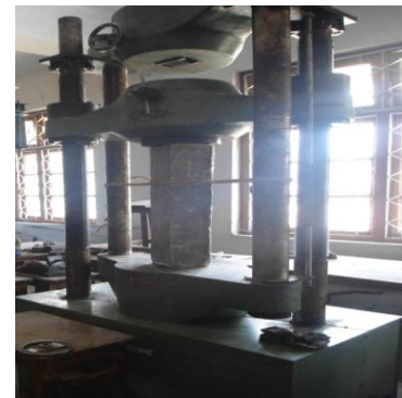
Figure 3. Complete test set up in UTM
