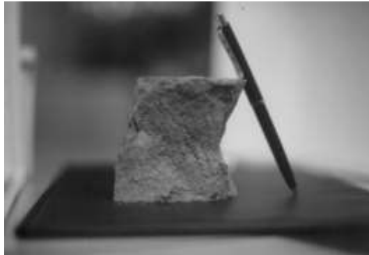
Figure 2. Compressive test and tested cubic adobe sample
