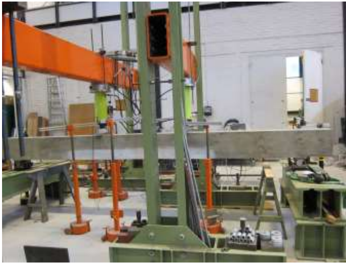
Figure 4. Concrete beam strengthened with pre-stressed CFRP laminate under four point bending test
