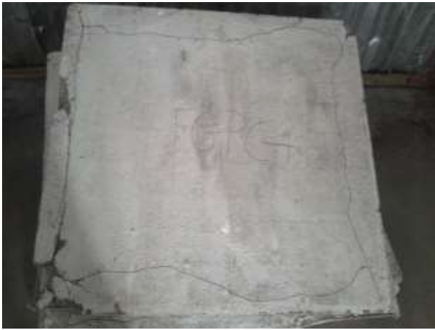
Figure 10. Negative yield line pattern
