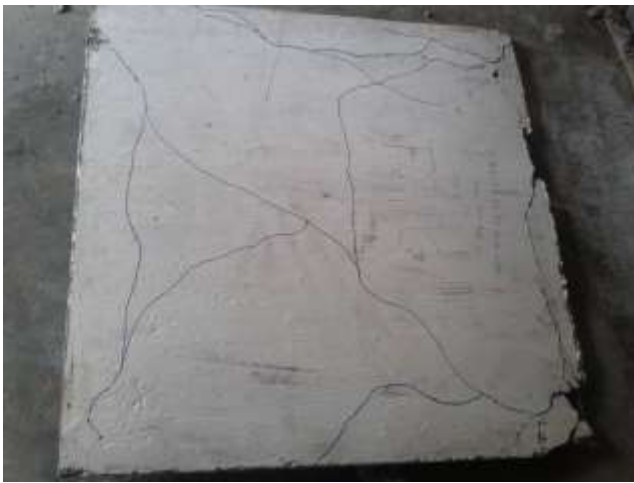
Figure 11. Positive yield line pattern
